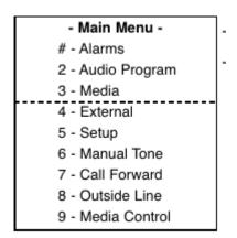
The phone will only display the top 3 (above the dotted line). In order to scroll up and down through the menu, press the (up / down) buttons.
